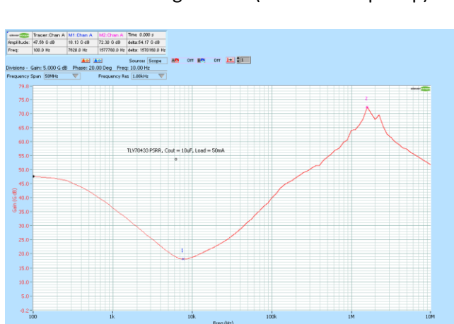
TLV70433 PSRR using CS1070 (1A 50 MHz op-amp):
